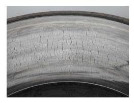
NOTICE: These classifications are made based on the worst area of the brake drum that is affected by heat check. It does not need to be visible completely around the braking surface. For example: If a drum has localized heavy heat check in an area that is approximately 6 In. across, but the rest of drum has no apparent heat check; the classification of this drum would be HEAVY.
