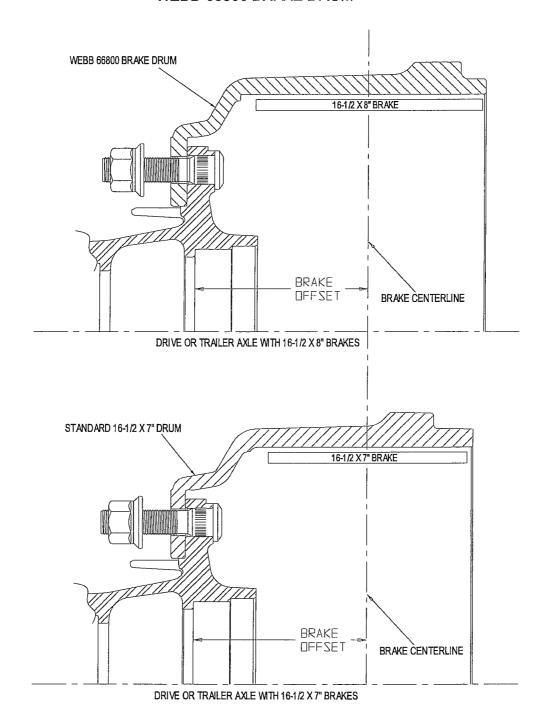
The Webb **66800** brake drum allows end-users to upgrade existing  $16-1/2 \times 7$ " brake shoe applications to  $16-1/2 \times 8$ " wide brake shoes without hub or brake spider modifications. This applies to standard Webb 2000-series universal hubs on R-series drive axles, TN-series trailer axles and TP-series trailer axles.
