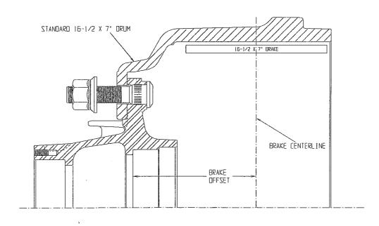
The Webb 66842 Brake Drum allows end-users to upgrade existing 16-1/2 x 7" brake shoe applications to 16-1/2 x 8-5/8" wide brake shoes without hub or brake speeder modifications. This applies to standard Webb 2000-series 8-stud hubs on R-series drive axles, TN-series trailer axles and TP-trailer axles.
