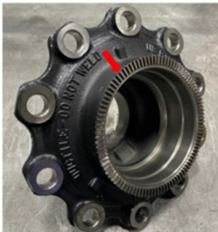
Direct machined ABS tone ring
