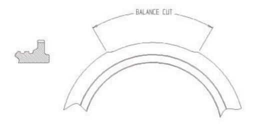
This change will be phased in over the next six (6) months starting July 5, 2003. This change will enable us to balance transit bus drums more efficiently and to improve this product by eliminating the welding of steel weights to the outside of the drum.
