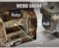
The patent-pending Webb design features a stainless steel clip that adds a protective barrier between the rotor and hub.
